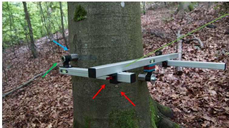
Loosen the clamping screws and the drill sleeve on the Align platform bolt .
