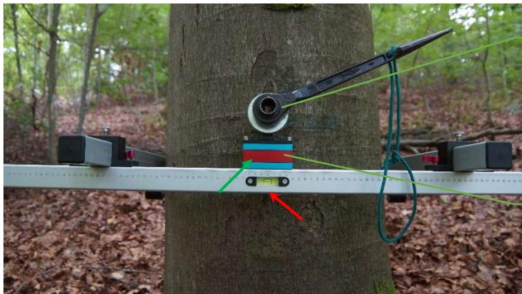
Attach the drilling device. Align using the **spirit level** and tighten with a nut and washer.
