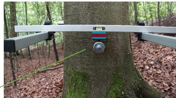
The drilling device is now in place upside down.
