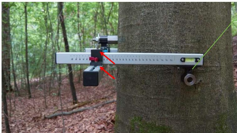
The drilling device has an axis spacing of 10 cm. Here in the picture, with **shims** 14 cm.
