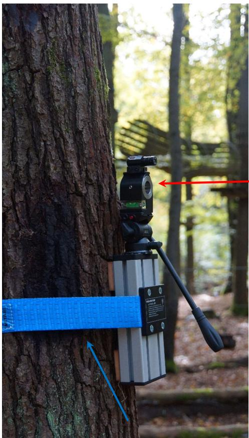
Secure the laser drilling jig with a lashing strap.
