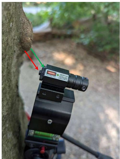
To insert the LR44 batteries, the power button **must be opened using the knurled screw** and closed again after insertion.
