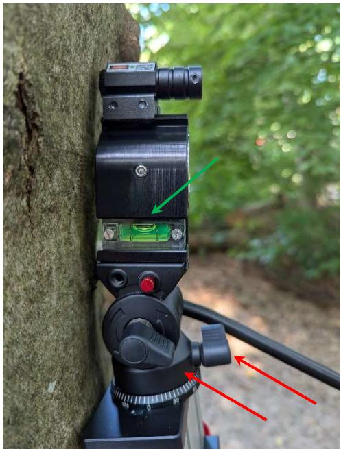
After releasing the two clamping levers, the laser can be aimed at the target tree and the drill sleeve can be placed into the water.
