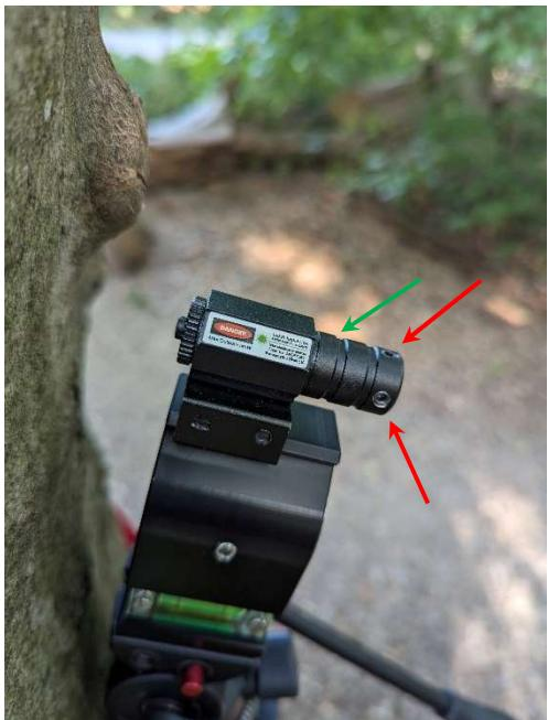
Calibrating the target laser using a construction laser.
