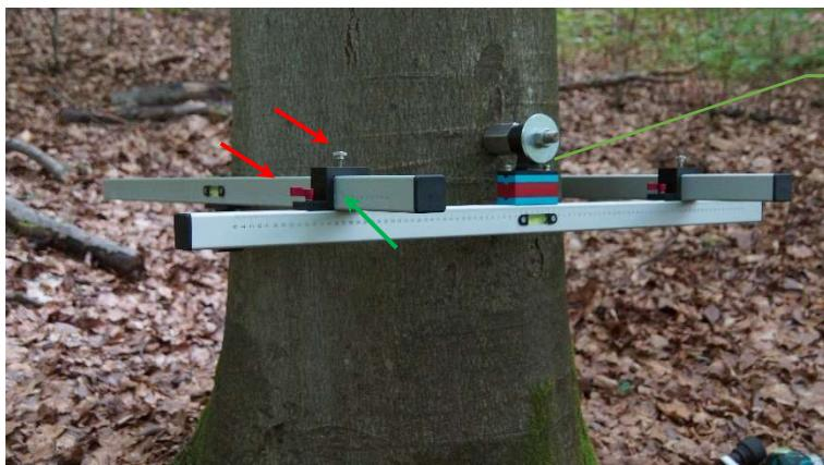
Loosen the clamping screws and slide the second arm to the read position with the help of the scale .
