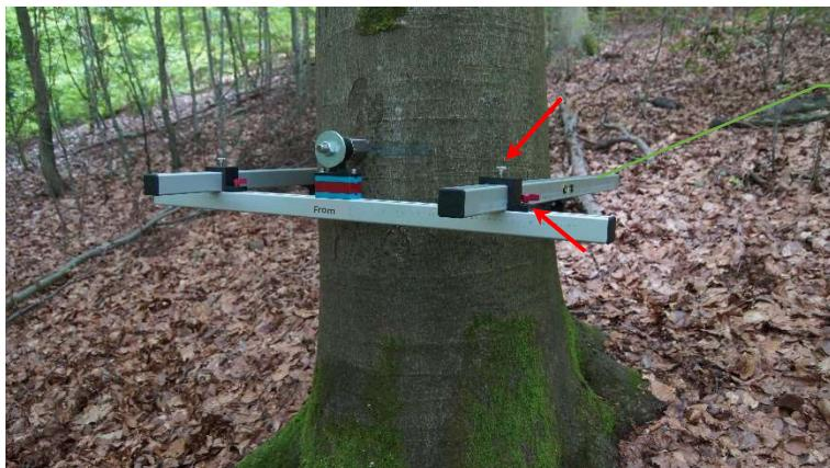
The drilling device has an axle spacing of 10 cm. Here in the picture, with **spacers** 14 cm.
