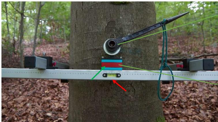
Attach the drilling device. Align using the water level and tighten with the nut and washer.
