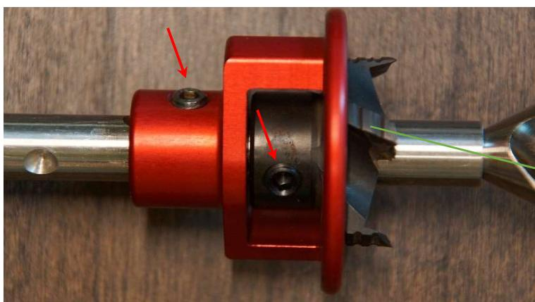
Set the position of the countersink and the depth stop, depending on the screw type.
