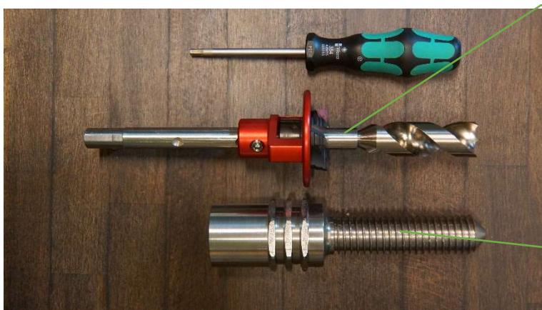
**IMPORTANT:** before tightening the two hex screws, align the surface of the drill shaft (hex) perpendicular to the two hex screws.
