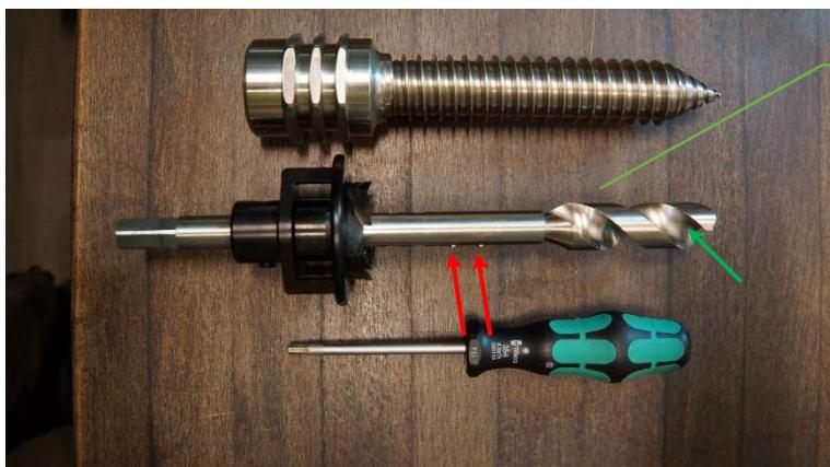
Select the drill diameter  $th$  that matches the screw.
