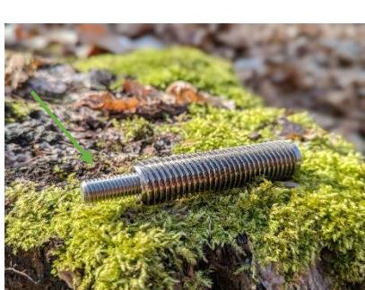
2.6.5 For softwood, installation with RAMPA sleeve type SKL, stainless steel 1.430 5, D 18.5, d M10, L 80mm is optionally recommended. ETA-12/048 1
