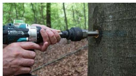
2.3.6 Position the bolt horizontally with a battery-powered screwdriver
