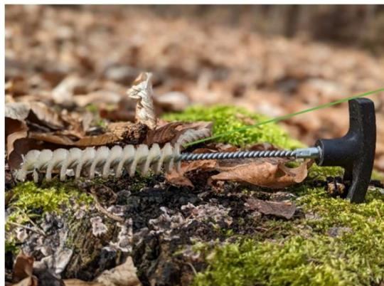
hole brush Ø suitable for the drilling. Used to remove wood chips from the drill hole.
