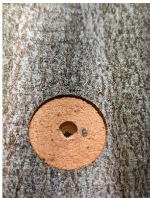
2.6.1 Drill a smooth surface using a picket drill Ø 40mm.
