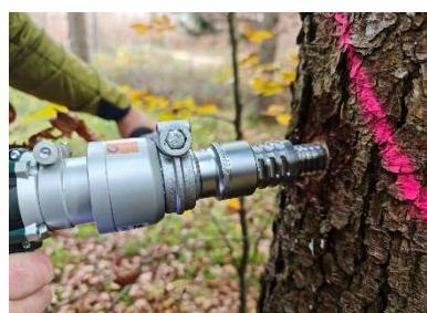
2.3.9 Screw in the bolt with a cordless screwdriver + torque multiplier.
