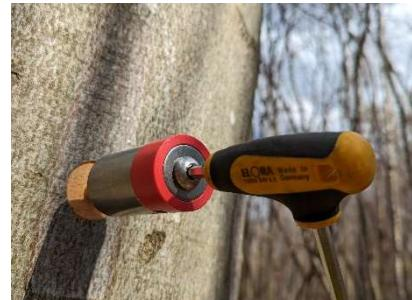
2.6.4 Screw in the rope carrier with an Allen key SW6.
