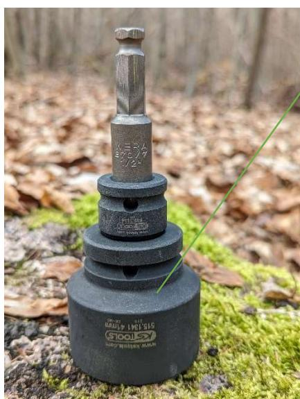
Socket wrench SW 41 with reducer and adapter for mounting the tree bolts.
