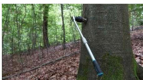
2.3.7 Drive the bolt with the telescopic ratchet into the final position.
